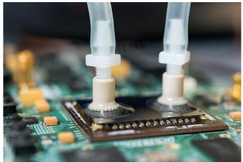
Initial tests involved "popular" 28-nanometer chips from Altera, and show promising results-- the researchers say "monolithically-cooled" chips operate at temperatures 60% below those of similar air-cooled chips. The aforementioned microfluidic passages are 100 microns in diameter and just few hundred microns away from the chip transistors. A silicon layer seals the fluid passages (except for an inlet and outlet), which carry regular de-ionised water.
