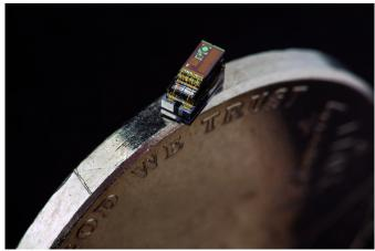
The result of 10 years of work by University of Michigan researchers, the M^3 is rather capable despite its minuscule dimensions. It can take pictures, read temperatures, record pressure and even communicate with other computers via radio. Such capabilities make it a "complete" computer.
