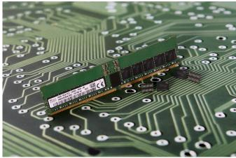
The next-generation DDR5 standard promises increases in both speed and density compared to DDR4, while reducing power consumption. SK Hynix says DDR5 memory consumes 30% less power than DDR4, and features a lower operating voltage set between 1.1 and 1.2 V. In performance terms, the 16Gb RAM claims a data transfer rate of 5200Mbps, 60% faster than 3200Mbps DDR4 RAM. The result, according to the company, is DRAM able to process 41.6GB of data per second.
