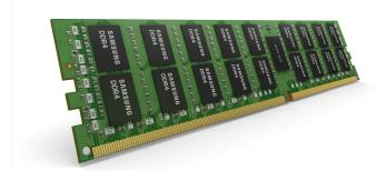
Bearing the model number M378A4G43MB1-CTD, the 32Gb UDIMM is rated to operated at DDR4-266 data rates at the standard 1.2V. Samsung does not provide timings, but they probably use standard JEDEC latencies for DDR4-266, being CL17 17-17 or higher. The chips are arranged as (2Gbit x 8) x 16. The modules are built using a 10nm process, and promise to be more energy efficient than Samsung DIMMs using a larger number of 8Gb devices.
