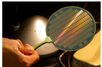
First described in a Nature paper, the CNT computer consists of 178 logic gates, can count up to 32 and performs counting and number sorting tasks. It runs code written in MIPS, fetching instruction from memory before execution at a clock rate of 1KHz.
