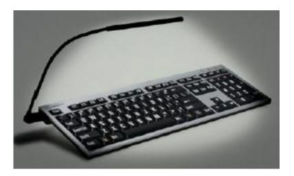
The LogicLight 2 features a touch sensitive on-off and dimmer switch. Just tap the tip end of the light with your finger and it goes on, off, or half power. The Logiclight is made up of 10 cool white LEDs with a heat temperature rating of about 4500. At half power, only 5 LEDs light up. The light shade can be rotated a full 360 degrees. The flexible light arm can be adjusted to any desired angle.
