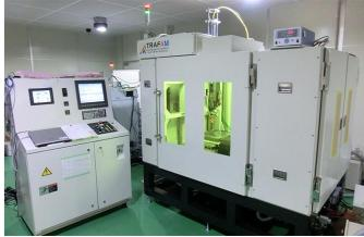
The printer uses laser metal deposition (LMD)-- a technology that deposits powdered metal and fires a laser beam in tandem. A high-speed nozzle based on Toshiba fluid simulation technology reduces the area where metal particles are injected, while the laser focuses very precisely on the tiny powder-covered area.
