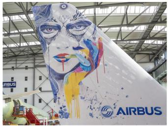
Painting a plane is something of a tricky business, one involving either a time-consuming process of multiple paint layers or the sticking of, well, giant stickers. The Airbus method promises to make the process a lot simpler via direct inkjet printing.
