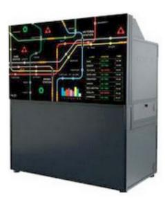
Christie's new **Entero LED 70**" **video wall display cube system**, shown at InfoComm, is an LED stackable display in a 16:9 form factor that features snap-in service panels, an improved mirror alignment system for precise mirror/geometry control and improved cosmetic features (it looks better).
