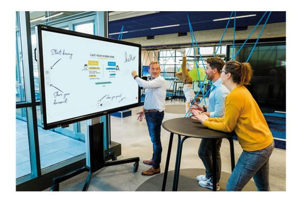
Like most with most collaboration devices, users can share content on the Leddura 2Share Pro using either the company app or a web browser and on-screen code. The board also features an integrated Barco ClickShare receiver, allowing users to share content using any ClickShare button. The display handles 3840x2160 resolution, and includes integrated 80W JBL speakers and far-field microphones with echo-cancellation technology.
