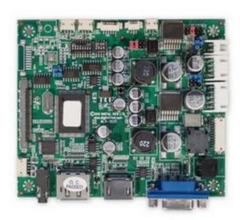
Designed for specialist monitor manufacturers and OEM display integrators, Digital View's ALR-1920 is a 1920x1200 (WUXGA), LCD Interface Board that supports HDMI, VGA and Display Port input for all small and large format HD LCD displays.
