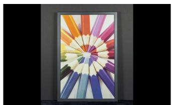
Described as a first in electrophoretic displays (EPD) ACeP achieves full colour gamut, including all 8 primary colours, without need for a colour filter array (CFA). The colour display uses a single layer of electrophoretic fluid controlled via voltages compatible with TFT backplanes. Such a solution is described as more commercially viable than alternative solutions involving complex stacked backplane structures.
