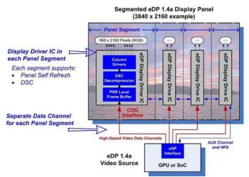
It incorporates the VESA Display Stream Compression (DSC) standard 1.1, as well as a segmented panel architecture allowing for higher panel integration.
