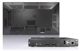
The OPS Slot-in-PC is an embedded computer able to support uses ranging from static content playback to demanding, interactive and high-resolution applications. It can handle anything from retail and digital-out-of-home (DooH) advertising to food and beverage menu boards, transportation wayfinding and information screens and digital cinema posters, among other use cases.
