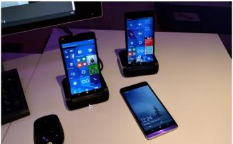
As one might (rightly) assume the Elite x3 makes heavy use of Continuum, the Windows 10 feature providing users with a PC-style experience on a smartphone through connection of a larger display, keyboard and mouse. Thus HP provides a pair of optional accessories for such purposes, the Desk Dock and the Mobile Extender.
