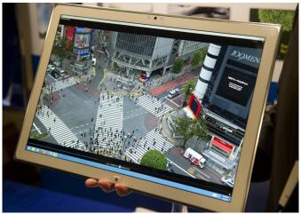
The device now carries an Intel Core i7-5600U v Pro processor and an AMD FirePro M5100 GPU, while the OS of choice is either Windows 10 Pro or Windows 7 Professional HDMI 2.0 input with support for Digital Cinema 4K (4090x2106@60fps) allows videographers and photographers to use it as a 20-inch 3840x2560 resolution viewfinder, as well as mobile workstation.
