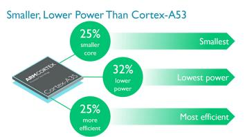
The Cortex-A35 features big.LITTLE configurability, supports 32- and 64-bit capabilities and is 25% smaller than the Cortex-A53. It also consumes less power (90mW per core according to ARM) while featuring enhancements such as a redesigned instruction fetch unit, new in-order 8-stage pipeline and improved NEON floating-point performance, making it ideal for next generation low-cost devices.
