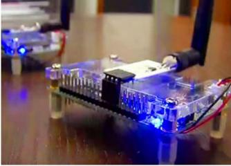
For the curious Passive Wifi energy consumption reaches up to 49.28  $\mu$ W when pushing 11Mbps transmissions. Energy use is even lower during 1Mbps transmissions, being around 14.48 $\mu$ W. According to the researchers such a rate is 1000x lower than Bluetooth LE and ZigBee, or 10000x lower than existing wifi chipsets.
