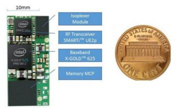
It features a SMART I UE2p transceiver, an Intel design combining transmitter and receiver functionality with an integrated power amplifier and power management on a single chip.
