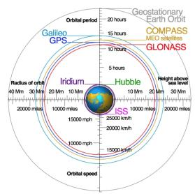
Internet services by satellite are widely available today from operators such as Astra and Eutelsat, operating in geostationary orbits at approximately 36,000 km altitude. At a rather lower level, the Iridium satellite network offers a global network from about 800km height, and is widely used for satellite phones and maritime services. Google is reported to be looking at orbits of only 160 km high, with the potential to remove any notable lag for the connection.
