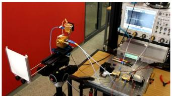
The wifi tests use 237.5GHz signals over a distance of 20m in laboratory conditions. However the super-high frequencies involved demand clear line of sight between devices at all times.
