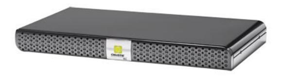
The Christie Brio is a totally wireless room system that allows up to five people to share their LCD or projection screens simultaneously. The output of Brio is two 2560?1600 (dual-link DVI-D — but can be converted to DisplayPort or HDMI) and stereo audio on 3.5 mm connectors. Inputs include up to two wired connections, five wireless inputs (from any resolution computer from 640?480 to 2560?1600 resolution), audio and all of it integrates support for HDCP.
