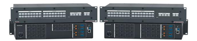
In addition, the switchers handle 4:4:4 colour sampling, HDR, Deep Color up to 12-bit, 3D, HD lossless audio formats and CEC, with technologies such as EDID Minder and Key Minder ensuring both system performance and compliance with HDCP-encrypted content. The matrix switchers also facilitate integration into a wide range of professional AV applications with audio de-embedding and audio breakaway capabilities.
