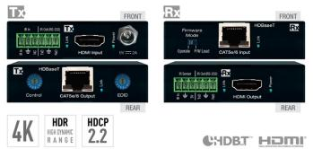
It can also extend signals up to 70m at 1080p/1920x1200 using CAT5e/6 cabling. The extender supports HDR10 at 4K 4:4:4, allowing users to experience a greater range of luminance levels. HDR10 delivery comes as part of the proprietary Full-Buffer Technology (FBT) a system managing TMDS re-clocking and signal regeneration, HDCP authentication to source and display, and EDID handshaking control.
