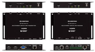
The package contains a 3x1+1 switcher, scaler and extender. The switcher has 2 HDMI inputs, 1 VGA input (with 1 analog audio input), and sends HDBaseT to the receiver mounted behind the room display or above the projector. The receiver features an additional HDMI input for a local source.
