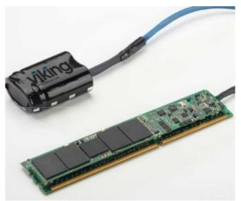
As a hybrid solution, the ArxCiv module leverages on the experience Viking has working on both DRAM and SSD technologies-- combining the speed and endurance of DDR3 memory with the non-volatile storage retention of flash memory.
