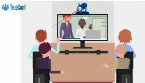
Tracker, well, tracks participants in a room through the combination of any UVC-compatible PTZ camera and the direction-finding Phoenix Audio Condor beam forming array. The Condor array divides the room into 7 sectors, and tracks voices in every sector using audio beams technology. In turn, the PTZ camera is voice tracked via microphone array beams by separating speakers in the conference room, and even includes additional coordinates such as tilt and zoom.
