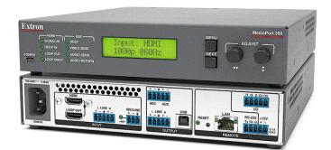
As the company puts it, the MediaPort 200 bridges between simple webcam-to-computer solutions and traditional hardware videoconferencing systems. It adds support for professional-grade equipment (such as videoconferencing PTZ cameras, boundary microphones and sound reinforcement systems) and easily integrates conferencing PCs into a fully equipped AV system complete with video distribution and processing, control, DSP, microphones and full sound reinforcement.
