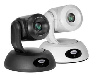
Vaddio builds on the RoboSHOT 30E NDI camera with the RoboSHOT 12E, a PTZ camera featuring NewTek NDI, the low latency technology allowing video systems to detect and communicate with each other over IP.
