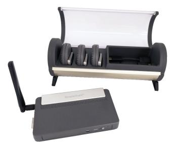
Designed as a cable replacement, SimpleShare is device-agnostic. It allows users to share HD video and sound wirelessly to any display with an HDMI input from any PC, Mac, DVD player, tablet, camcorder or other devices in real time. The system features simple plug-and-play installation with no software, downloads or network management, making it user-friendly to implement. Users can switch between up to 254 presenters with the click of a button.
