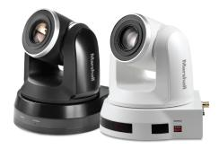
The camera is controllable remotely via RS323 over ethernet cable or RS422 over twisted pair, and uses common protocols for compatibility with most integrated control systems. It offers multiple outputs, including HD-SDI (3G) and HDMI (DVI), and many broadcast adjustable settings such as white balance, exposure, iris, gamma and black level. The pan-tilt range spans 340-degrees horizontally and 120-degrees vertically, with simultaneous 4D control of pan, tilt, zoom and focus.
