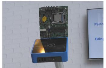
Named after their dimensions (5.5- x 5.8-inch, or 140 x 147mm), 5x5 motherboards have a 29% smaller surface area than the mini-ITX standard. The boards build on Intel's NUC mini-PC concept, and feature a land grid array (LGA) processor socket, two laptop-style SODIMM slots and storage in either 2.5-inch SATA or M.2 SSD form.
