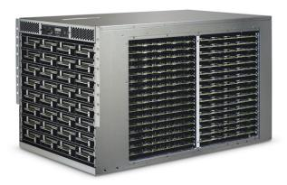
SeaMicro builds space- and energy-saving servers by using hundreds of "wimpy cores"-- ultra-low-power processors-- specifically Intel chips, including Atom and Xeon processors. The company will continue making servers using Intel chips (for now) before it transitions towards AMD-based solutions sometime around H2 2012.
