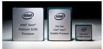
Previously dubbed "Cascade Lake," Xeon Scalable processors support Optane DC persistent memory, bringing support for up to 36TB of system-level memory capacity in combination with traditional DRAM. Turbo Boost 2.0 technology ramps up to 4.4GHz, alongside memory subsystem enhancements with support for DDR4-2933 MT/s and 16 Gb DIMM densities.
