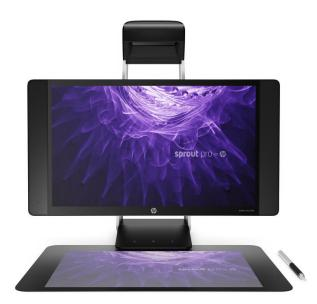
If one needs a refresher, the <u>Sprout is a "blended reality" PC</u> designed mainly for creative professionals. It looks like a regular AiO PC, if one with projector protruding from the main display. The projector has multiple uses, since it not only projects the aforementioned Touch Mat surface, it also acts as a scanner for both 2D and 3D objects.
