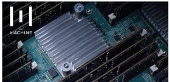
The Machine brings together a number of advanced technologies. As well as memory-driven computing it also includes photonics and a new fabric able to handle vast amounts of data. The aforementioned prototype involves compute nodes sharing a pool of fast and permanent Fabric-Attached Memory, operational photonics-based data links and a custom Linux-based OS running on a customised SoC.
