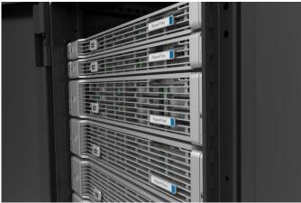
The HyperFlex system consists of a number of products, the first being the HXData Platform-- a co-development with storage software developer SpringPath using Cisco UCS servers to form a distributed storage system consisting of SSDs and HDs from federated storage clusters.
