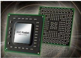
These APUs incorporate – in a single die design – multi-core CPU (x86) technology, a discrete-level graphics and parallel processing engine for DirectX 11, a dedicated high-def video acceleration block, and a high-speed bus (speeds data across the differing types of processor cores within the design).
