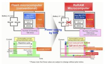
Also known as memristor or "memory resistor," ReRAM combines the properties of a resistor and memory in a new circuit element. Memristor technology requires less energy, is faster than present storage technologies and retains information even when the power is off.
