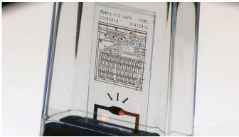
Designed to store critical data such as encryption keys, the chip is built using Gorilla Glass, the tough glass used in many smartphone displays. As PARC puts it the glass is "ion-exchange tempered," a process causing the glass to be stressed to the point where it can break through the application of heat.
