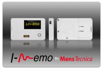
The I-Memo is a portable password-storing device smaller than a mobile phone, allowing access to stored passwords via fingerprint verification instead of a master password.
