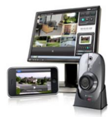
Both models carry a 720p camera (with 130-degree lens), built-in microphone, professional-grade wall mounts, 2GB MicroSD card (for storage) and free live remote viewing on PC, Mac or smartphone (via iOS, Android and Blackberryn apps).
