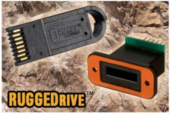
The company says it uses a solid over-moulding process for RuggeDrive memory tokens, with a tough composite plastic protecting internal components. This allows their use in harsh environments, such as military, industrial, commercial and medical settings.
