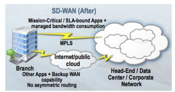
SD-WAN leverages hybrid WAN, and adds a centralised, application-based policy controller, analytics for application and network visibility, a secure software overlay (abstracts underlying networks) and an optional SD-WAN forwarder (routing capability). It allows for cost-effective application delivery, meeting the needs of modern branch/remote sites, optimising software-as-a-service (SaaS) and cloud-based services, and improving branch-IT efficiency through automation.
