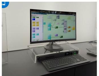
The successor to the Harvey mx.16 handles audio signal processing, lighting and media control, making it suitable for a number of different channels. The audio input and output channels are scalable in steps of 4, meaning Harvey variants can cover the requirements of a small project with an 8x8 audio matrix to special applications such as 4x24 channels.
