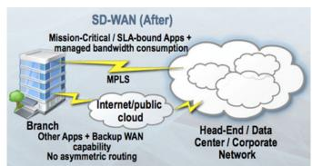
SD-WANs leverage hybrid WANs but incorporate a centralised, application-based policy controller, analytics for application and network visibility and security, a software overlay to abstract underlying networks and optional routing capability providing intelligent path selection across WAN links. It provides means to optimise cloud/SaaS applications while providing a dynamic and secure WAN fabric for distributed enterprises.
