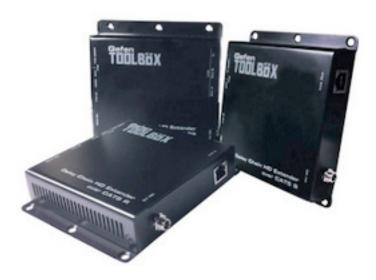
Gefen's **Daisy Chain HD System** creates a large infrastructure for wiring displays using CAT-5 cable. The system includes sender, splitter and receiver units—all interconnected in a daisy chain concept. All three units work together to extend 1080p full HD with RS-232 and IR control signals using the same CAT-5 cable.
