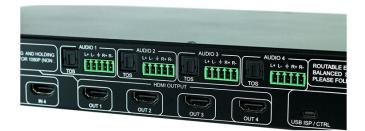
The switch claims to equalise and amplify the output to ensure the HDMI signal can be transmitted through long HDMI signals without quality loss. Meanwhile built-in 1080p to 4K and 4K to 1080p scaling on each output allows for EDID management. Fully matrix-able audio allows one to move the audio signal independently from the video signal at any of the de-embedded audio outputs.
