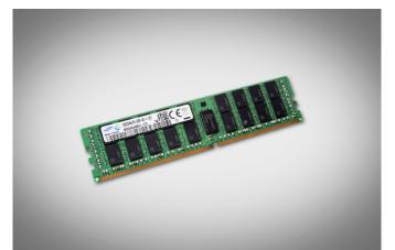
An update on the 64GB TSV DDR4 DRAM modules introduced in 2014, the new Samsung TSV DRAM modules claim the largest capacity and highest neergy efficiency around, while offering high speeds and "excellent" reliability. Each 128GB TSV DDR4 RDIMM carries 144 DDR4 chips arranged into 36 4GB DRAM packages. Each package in turn contains four 20nm-based 8Gb chips assembled using TSV packaging technology.
