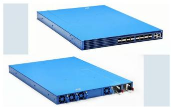
Announced back in June 2014, the Wedge was designed as a more flexible and scalable alternative to traditional switches. It works with both commercial and open-source networking products and packs an actual microserver module (one based on Facebook's "Group Hug" architecture), meaning it runs a server complete with own networking OS next to the traditional networking silicon.
